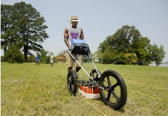
Staff photo by Thomas J. TurneySumer intern from Norfolk State Kevin Brodie II uses a ground penetrating radar to survey an historic site on Rivershore Road, Thursday, June 21, 2012.
